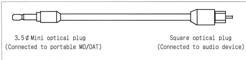
Fiber-Optic Cable Schematic Diagram
