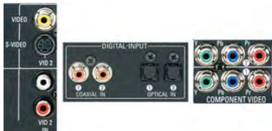
Figure 18 – Video 2 AV, Digital Audio and Component Video Inputs
