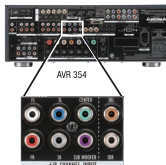
Figure 21 – Connecting a Multichannel Audio Player
