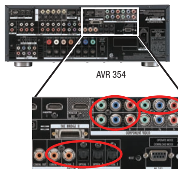
Figure 22 – Connecting a Component-Video-Equipped Disc Player
