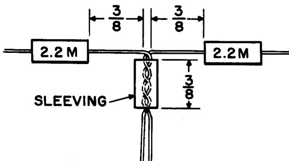
4) Connect the twisted leads of the pair of 2.2 megohm  $\frac{1}{2}$  watt 10% resistors (red, red, green, silver) through the loop of SD1 and SD2 (S). Cut off excess wire. Connect one free end of the pair of resistors to T5 lug #1 (NS) and connect the other free end to T5 lug #2 (NS). See addendum pictorial, detail C.
