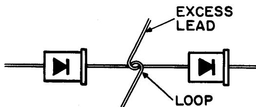
2) Change step 12 to read, "Hook anode lead from SD3 with cathode lead SD4 (NS). Do not cut off excess wire."
