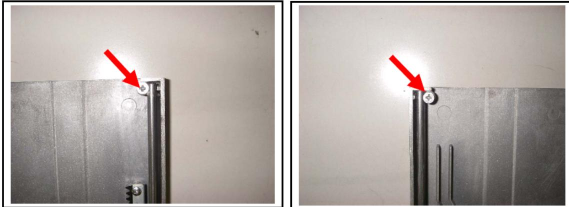
2) Take out the screws that hold the TRAY-SHAFT. (2 on each of the left and right sides.)
