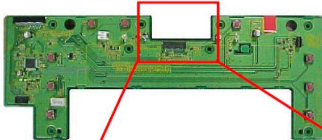
(3) Replace the POS. NO. RY10 with a CHIP RES. 62K OHM.
