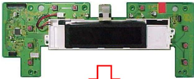
(2) Take the LCD unit off the PY16 (FRONT 1 PWB).
