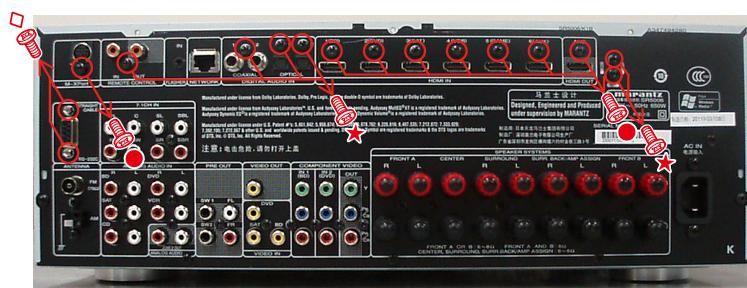
(2) Disconnect the connector board.
