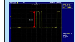
Example of waveform in check ② Voltage scale : 1.0V/div Time scale : 1us/div
