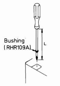
• If you attach a bushing (part number: RHR109A) to the tip of the screwdriver as shown in the figure, the screwdriver tip will easily fit in the screw heads and you will be able to remove the screws with ease.
