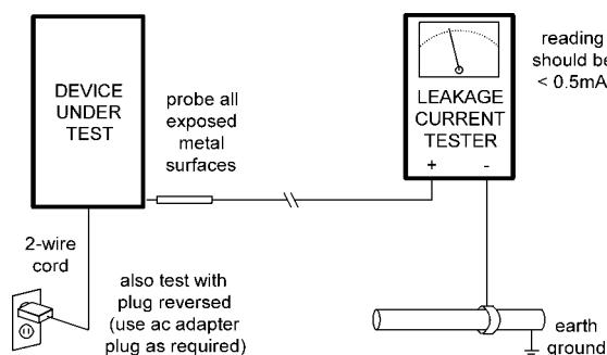
ANY MEASUREMENTS NOT WITHIN THE LIMITS SPECIFIED HEREIN INDICATE A POTENTIAL SHOCK HAZARD THAT MUST BE ELIMINATED BEFORE RETURNING THE INSTRUMENT TO THE CUSTOMER OR BEFORE CONNECTING TO ANTENNA OR ACCESSORIES.
