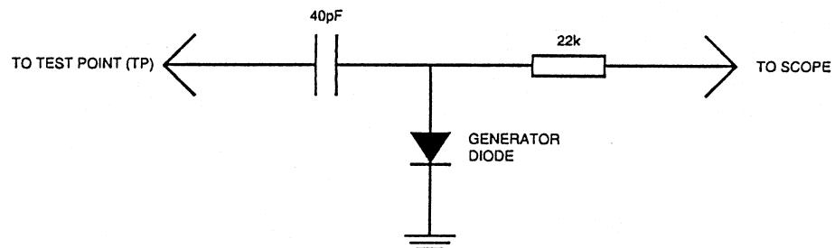
Figure 7. Alignment Pad #1
