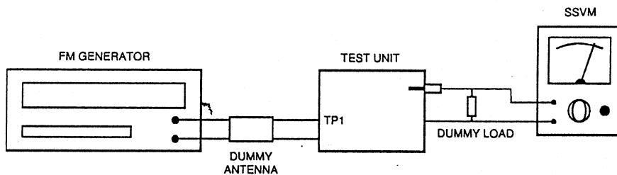
Figure 6. FM Band/Traking
