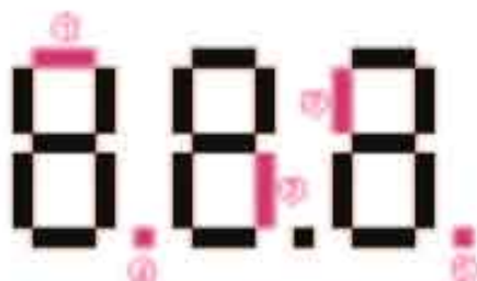
Fig. 45. 7 Lighting Sequence of Seg-LEDs
