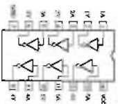
IC152: TC74VHC04AF1 Hex Inverters
